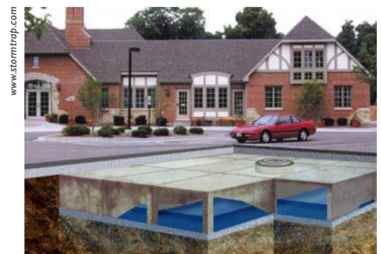
Underground storm water management systems
